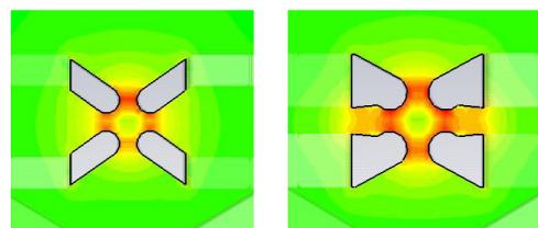
Figure 4: Field geometry of two different clamp heights.
