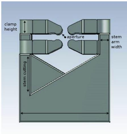
Figure 2: Parameter variations of the stem shape.
